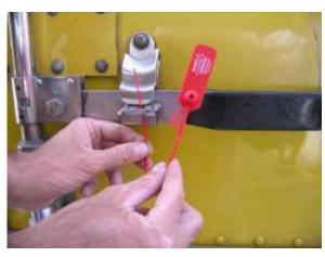
Insert the seal tail inside the door handle holes.
