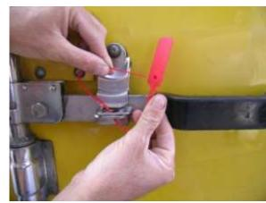
Insert the tail of the seal in the back hole of the seal head.
